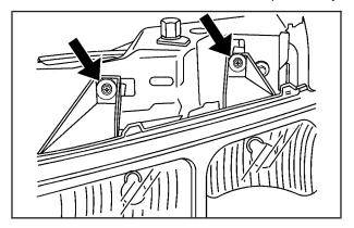
Remove the two pins on the top of the headlamp assembly. To remove the pins, turn the outer pin clockwise and pull it straight up. To remove the inner pin, turn it counterclockwise and pull it straight up.
